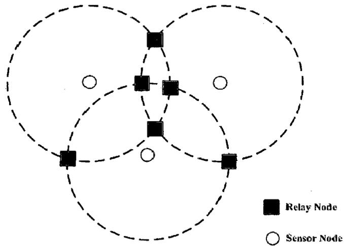
**Figure 3.2 Intersection based placement of relay nodes**
