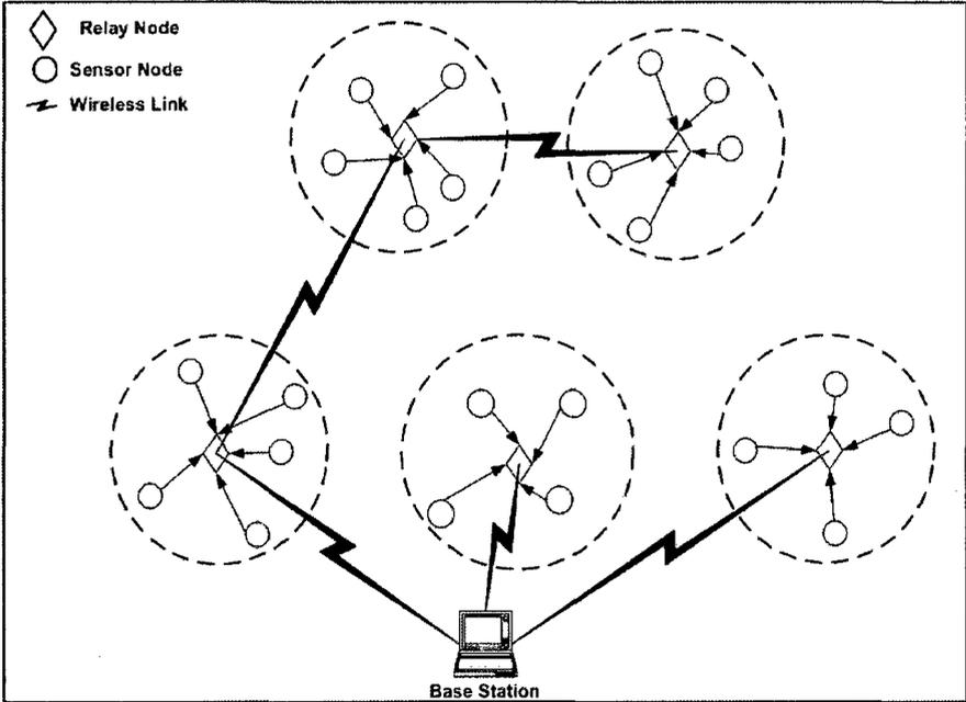
**Figure 2.4 Using relay nodes in hierarchical sensor networks**
