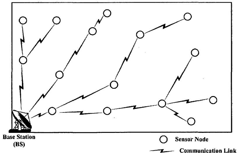
Figure 1.1 General layout of a sensor network
