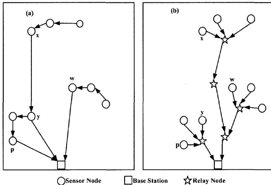
**Figure 2.3 Using relay nodes in flat sensor networks**
