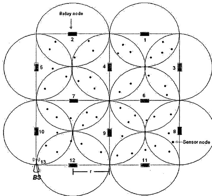
Figure 3.1 Grid based placement of relay nodes
