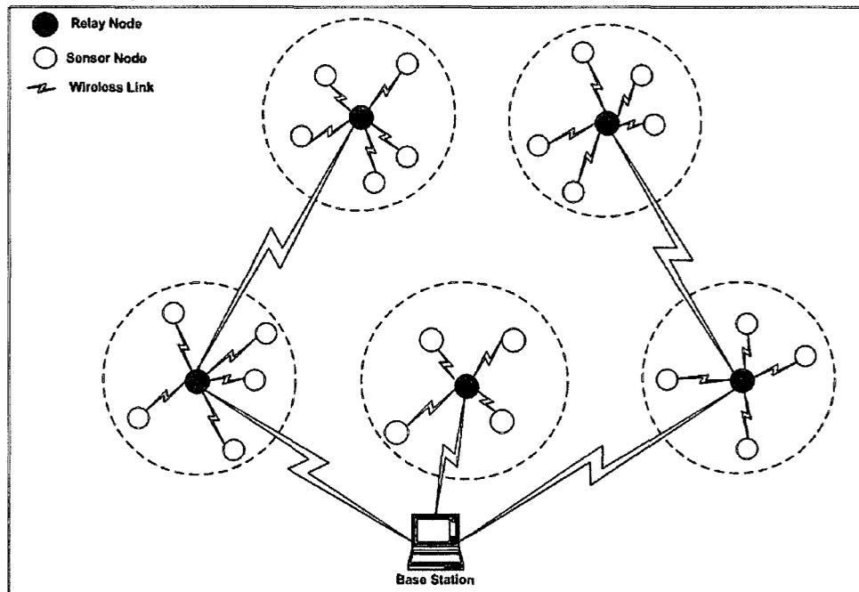
**Figure 1.2 General layout of a hierarchical sensor network**
