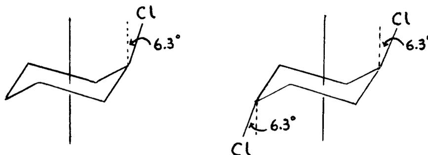
Fig. II-3. Ring deformation as shown by electron diffraction.
