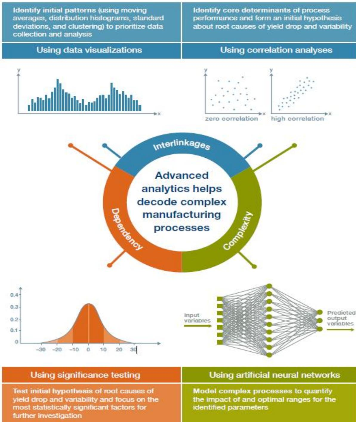
Figure 6. Advanced analytics for complex manufacturing processes (Auschitzky et al., 2014).
