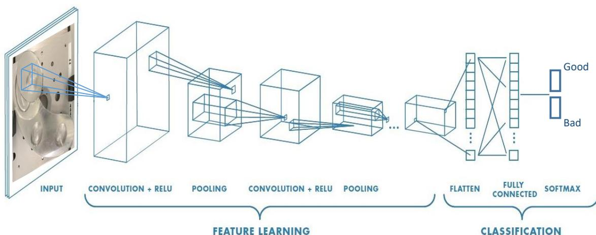
Figure 33. Structure of convolutional neural networks (CNN) (FreeCodeCamp, 2019).
