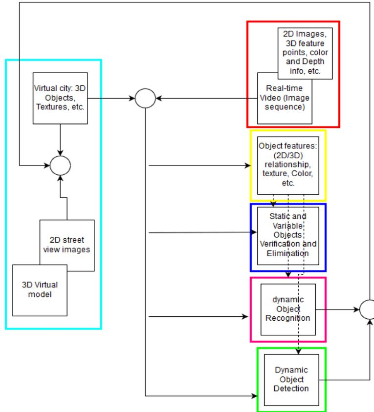
Figure 30: Overall system architecture
