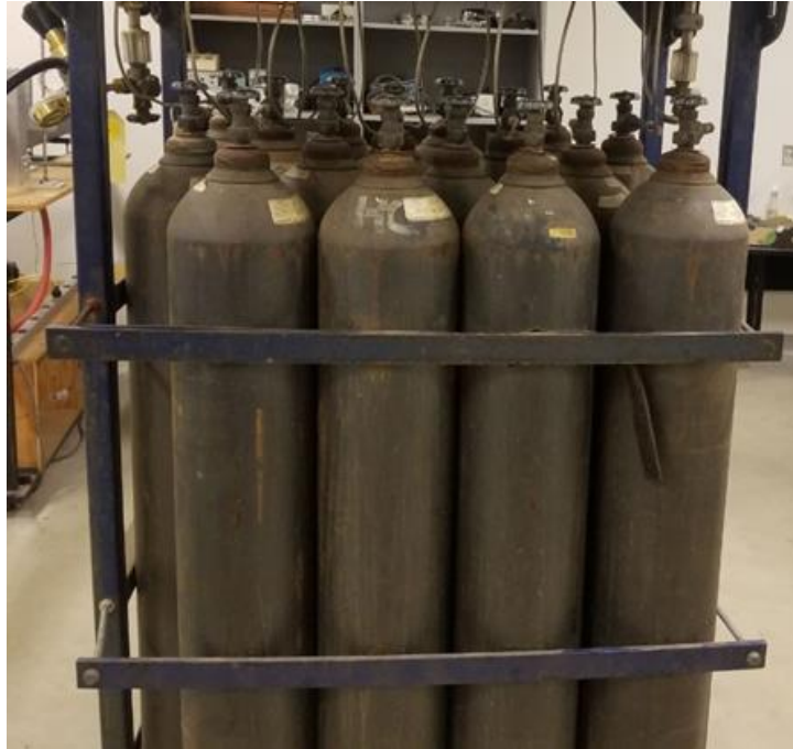
Figure 3.10: Pressurized N 2 tanks
