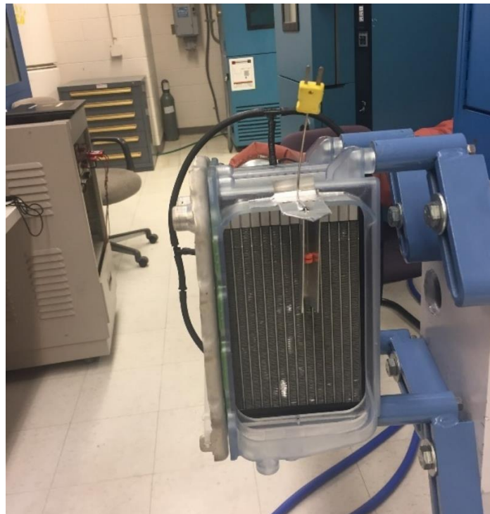
Figure 21: View of CSB outlet gutter/thermocouple
