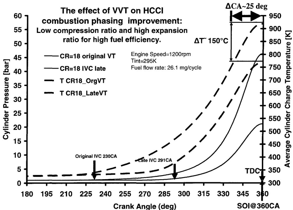
Figure 5.4 Pressure/Temperature Comparison between VVT and Original Valve Timing Case
