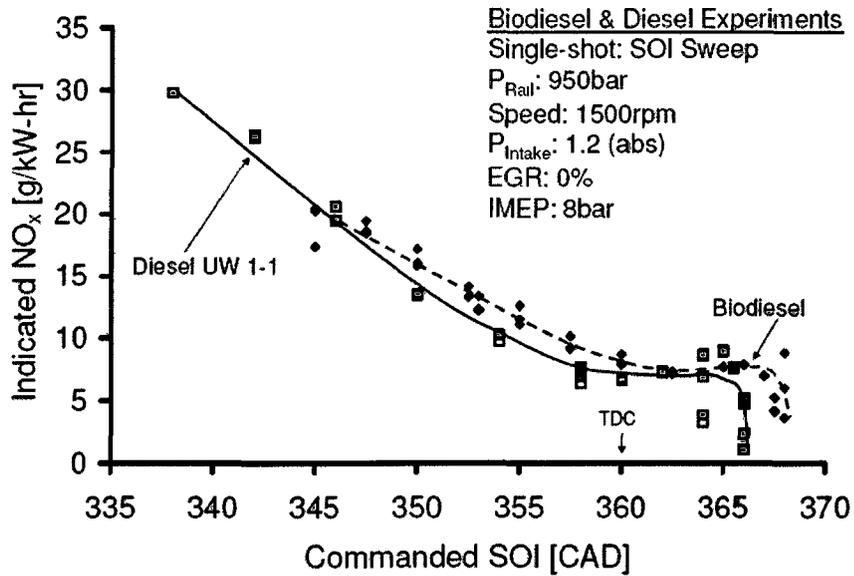
Figure 4.11 Comparison of the Injection Timing Effect on  $NO_x$  Emissions between Diesel and Biodiesel Fuels
