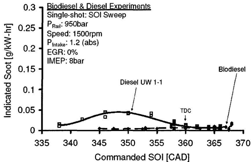
**Figure 4.12 Comparison of the Injection Timing Effect on Soot Emissions between Diesel and Biodiesel Fuels**
