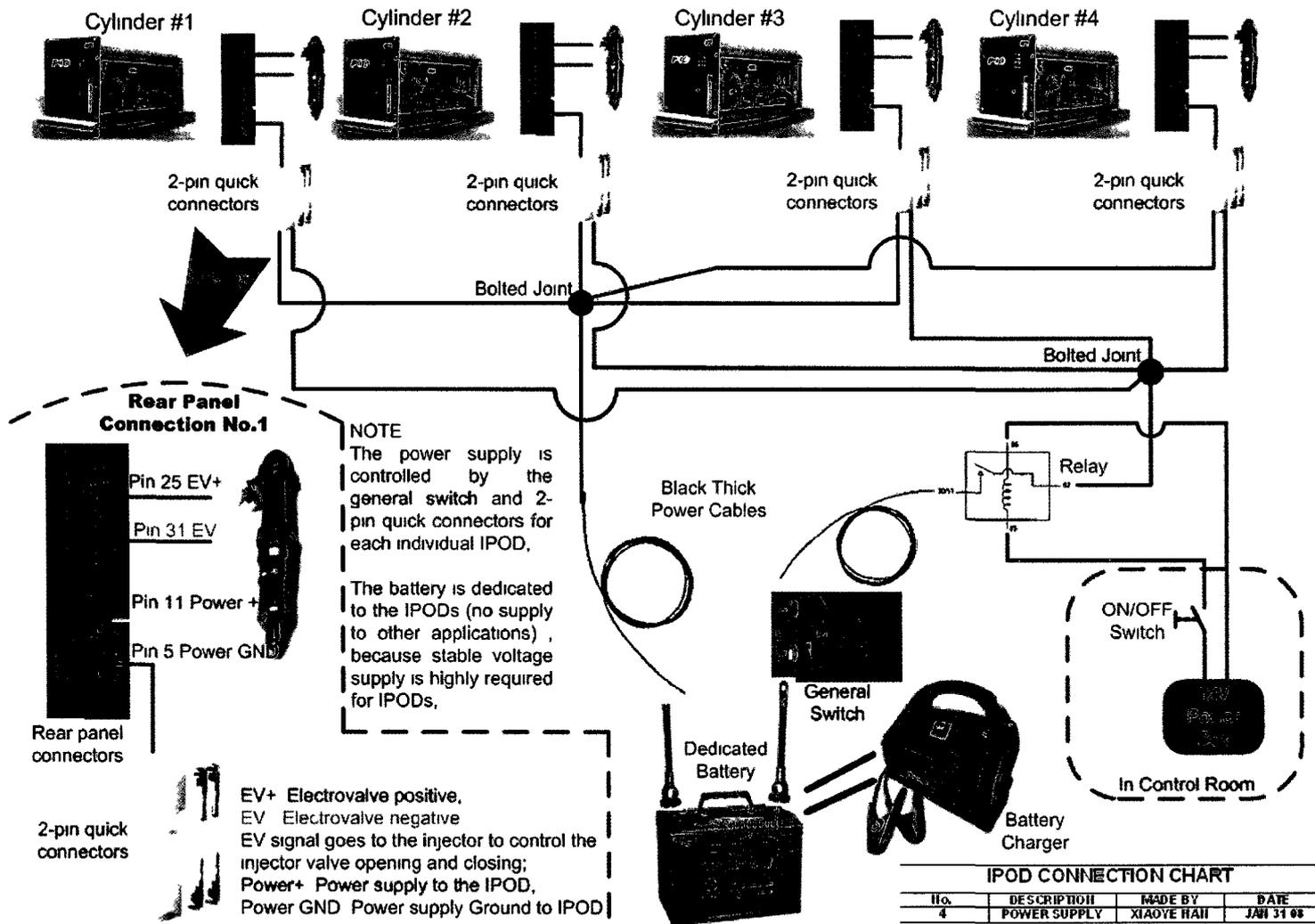
Figure 3.9 IPOD Power Supply Connections
