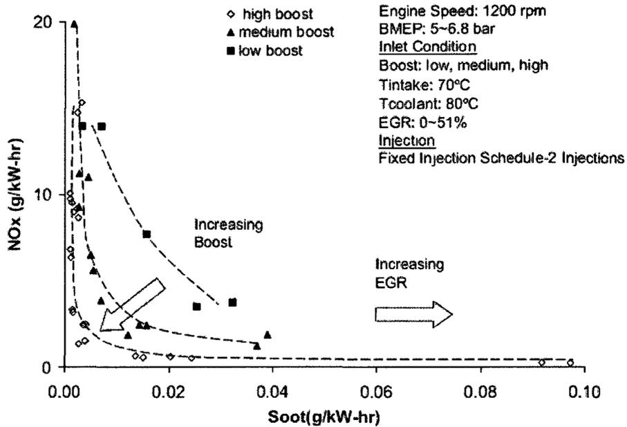
Figure 1.4 Boost and EGR Effect on NO<sub>x</sub>/Soot Reduction [5]
