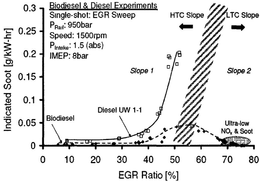
Figure 4.10 Comparison of the EGR Effect on Soot Emissions between Diesel and Biodiesel Fuels
