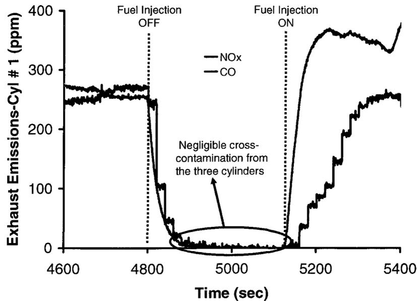
Figure 4.1 Exhaust Contamination Test
