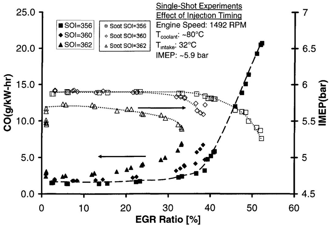
Figure 4.7 Effect of Increasing EGR on CO Emissions and IMEP
