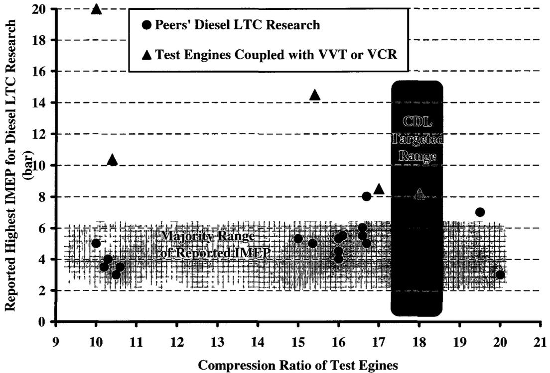
Figure 1.9 Load Range of Reviewed Peers' Diesel LTC Research according to Different Compression Raito [9~37]
