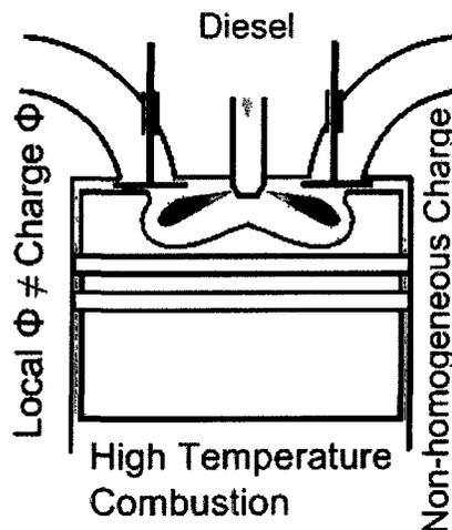
**Figure 1.1 Conventional Diesel Combustion**
