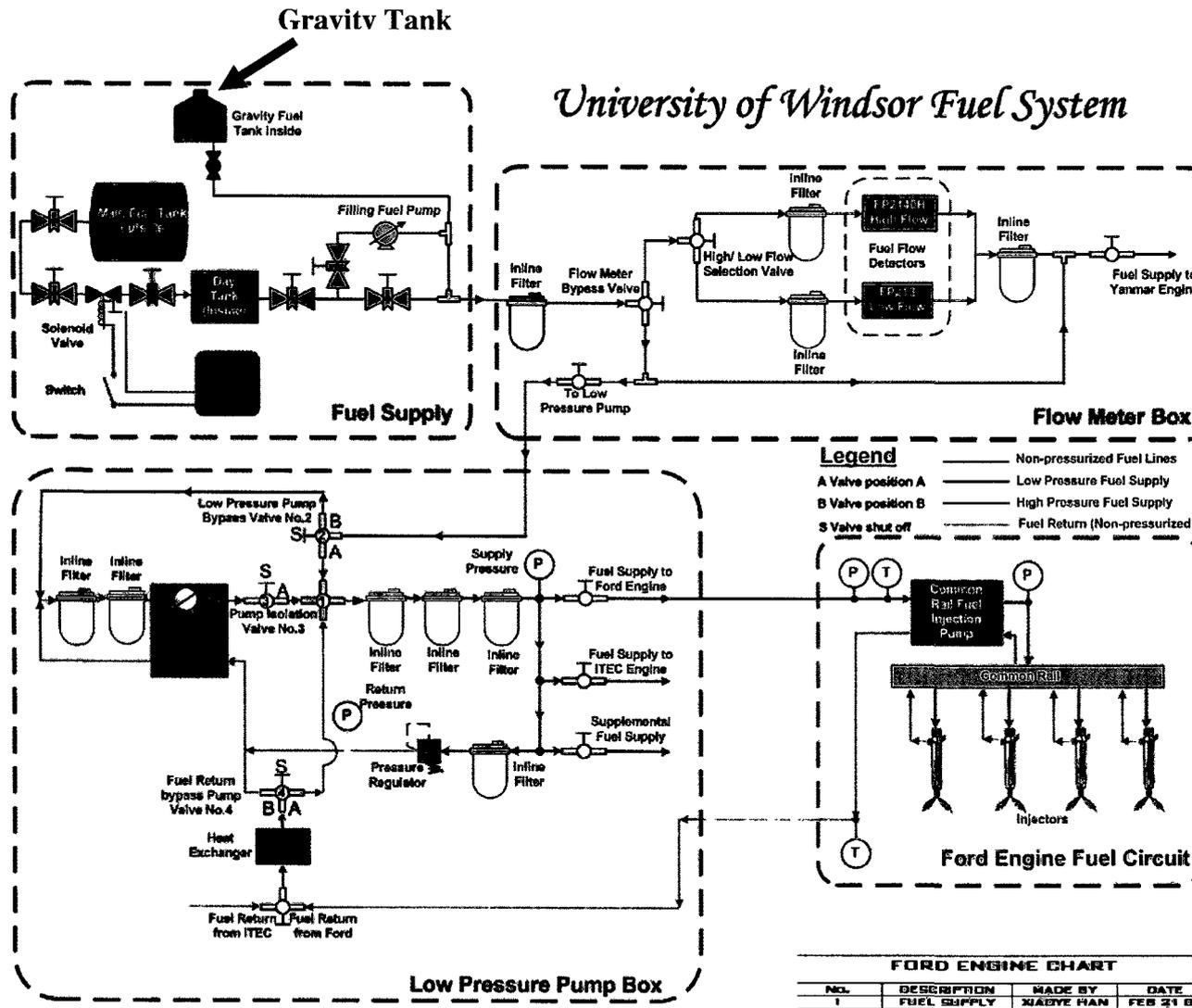
Figure 3.12 New Fuel Supply and Return Systems in the CDL
