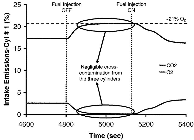
**Figure 4.2 Intake Contamination Test**
