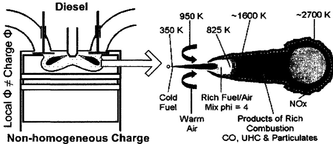
Figure 1.3 Diesel Fuel Spray and Flame (adapted from Flynn et al.) [4]
