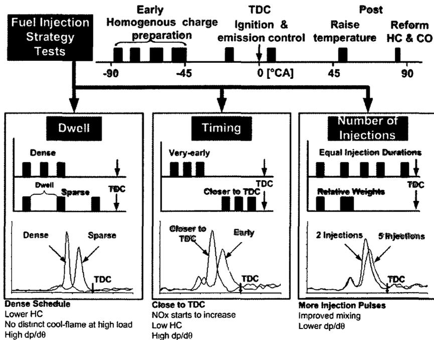
Figure 1.5 Injection Strategies for Diesel Combustion Research
