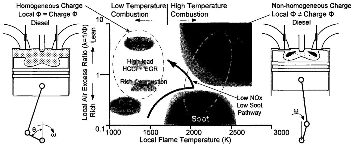
**Figure 1.7 Conventional Diesel Combustion and Low Temperature Combustion (Zheng et al. 2007e)**
