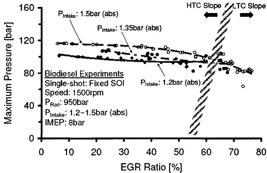
**Figure 4.13 Pmax with EGR under Different Boost for Biodiesel**
