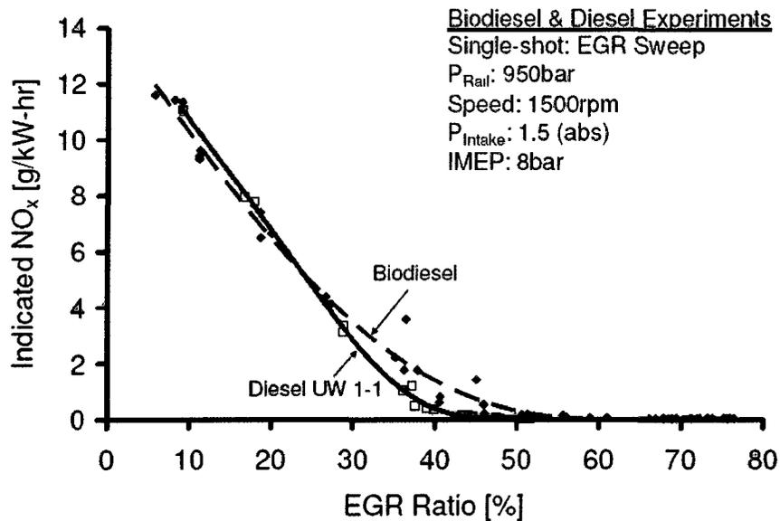
**Figure 4.9 Comparison of the EGR Effect on NO<sub>x</sub> Emissions between Diesel and Biodiesel Fuels**
