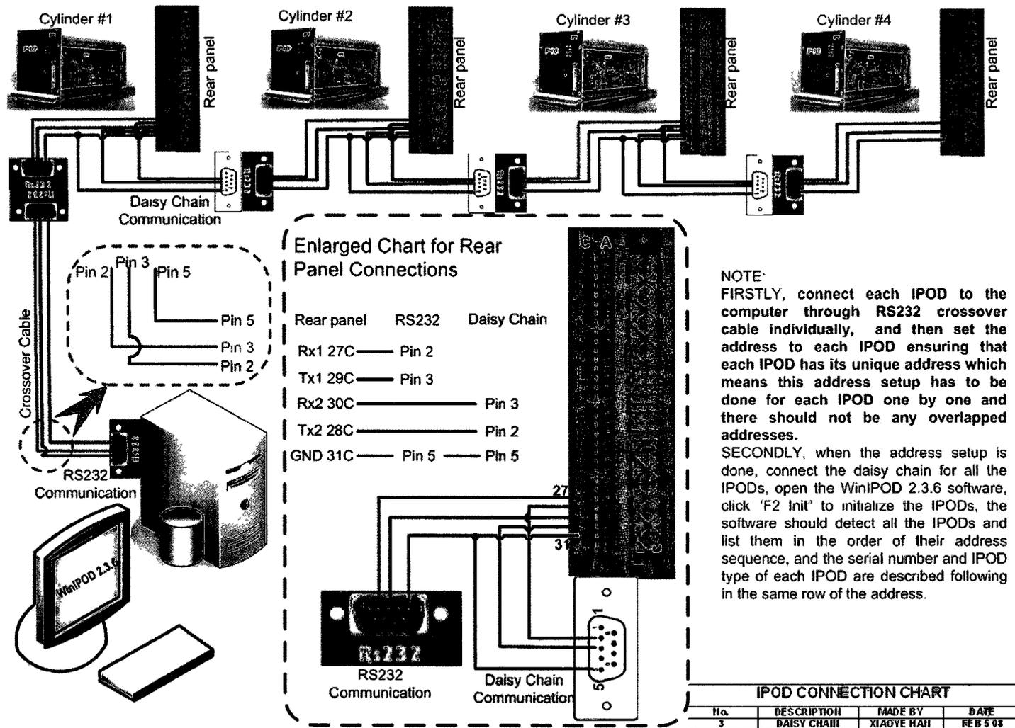
Figure 3.11 Daisy Chain and Communication Cabling of IPOD Drivers
