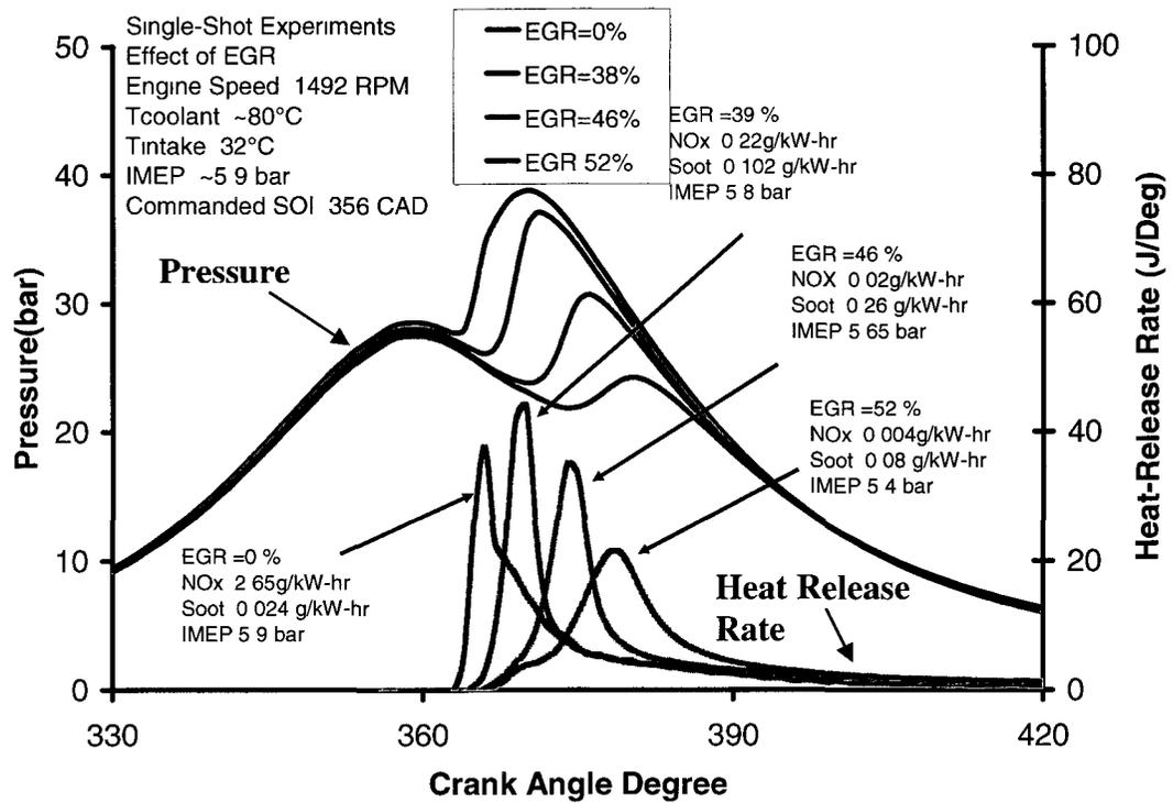
**Figure 4.8 Effect of Increasing EGR on Heat Release Rate**
