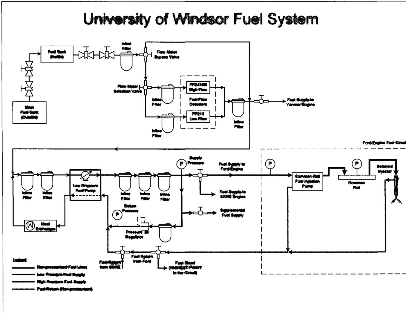
Figure 2.5 Original Fuel Supply and Return System
