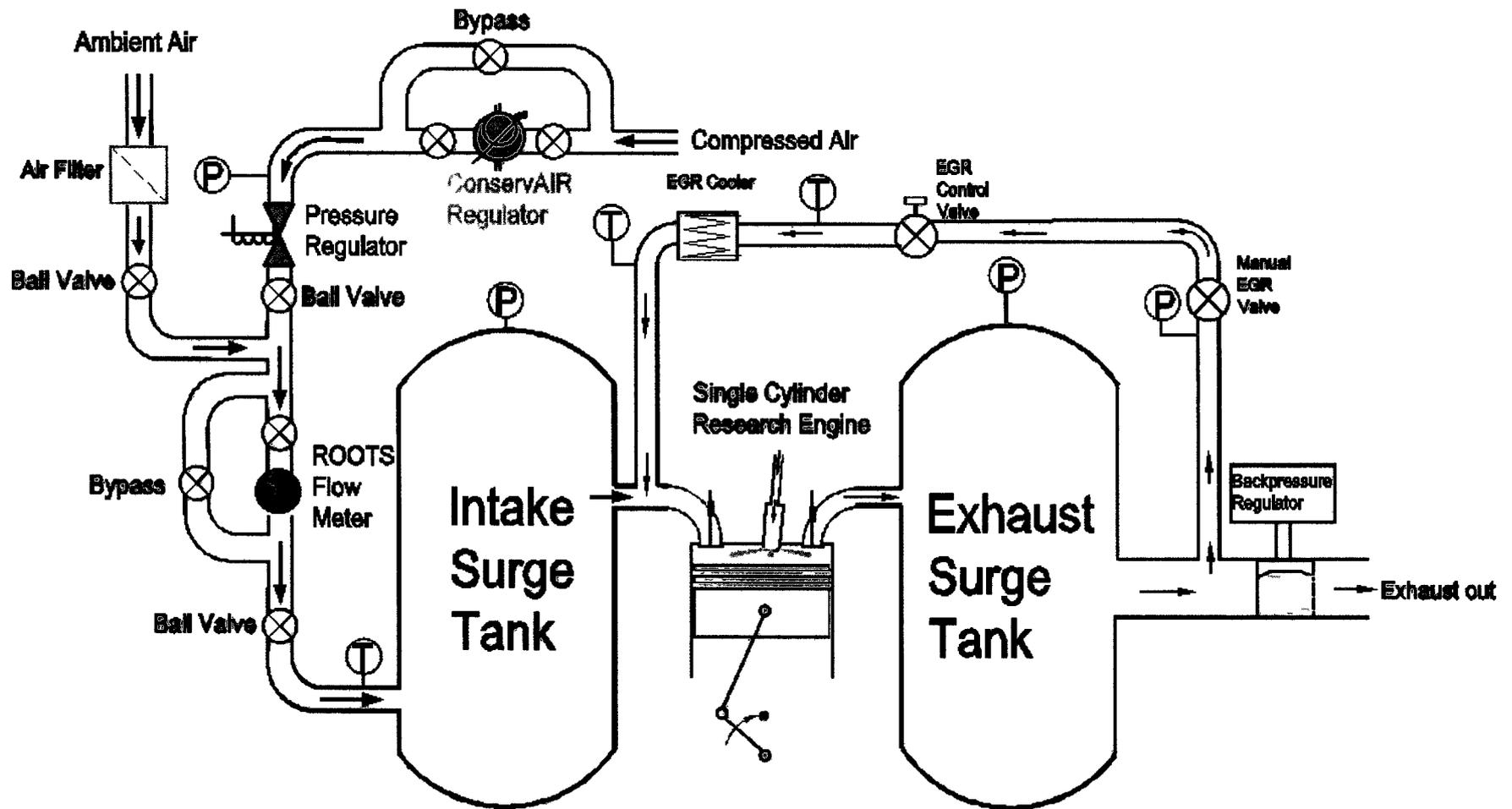
Figure 2.1 Intake and Exhaust Systems of Single Cylinder Research Engine in the CDL
