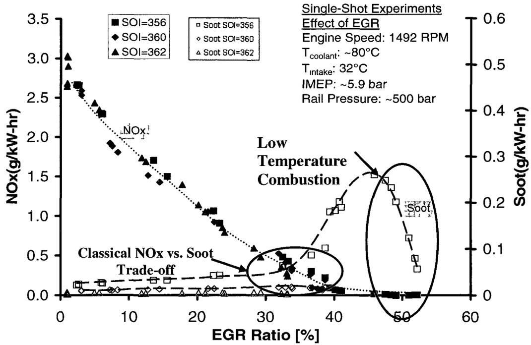
Figure 4.6 Effect of Increasing EGR on Soot and NOx
