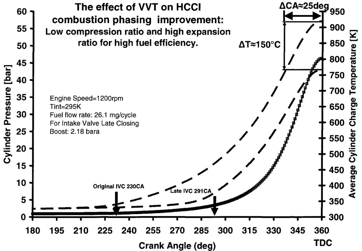
Figure 5.5 Pressure/Temperature Comparison between Boosted VVT and Original Valve Timing Case
