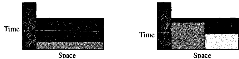
Figure 9. A group with poor utilization (Left) A group with better utilization (Right)
