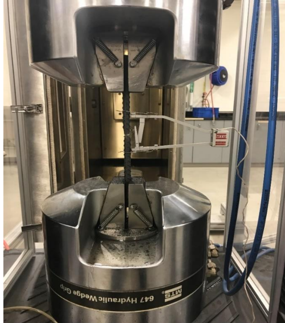
Figure 3.12: Steel rebar test
