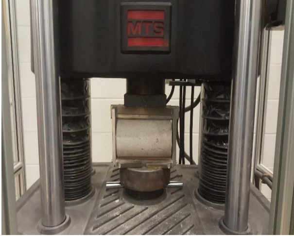
Figure 3.6: Split tensile test
