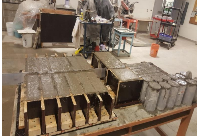
Figure 3.1: Casting of Specimen for Phase one
