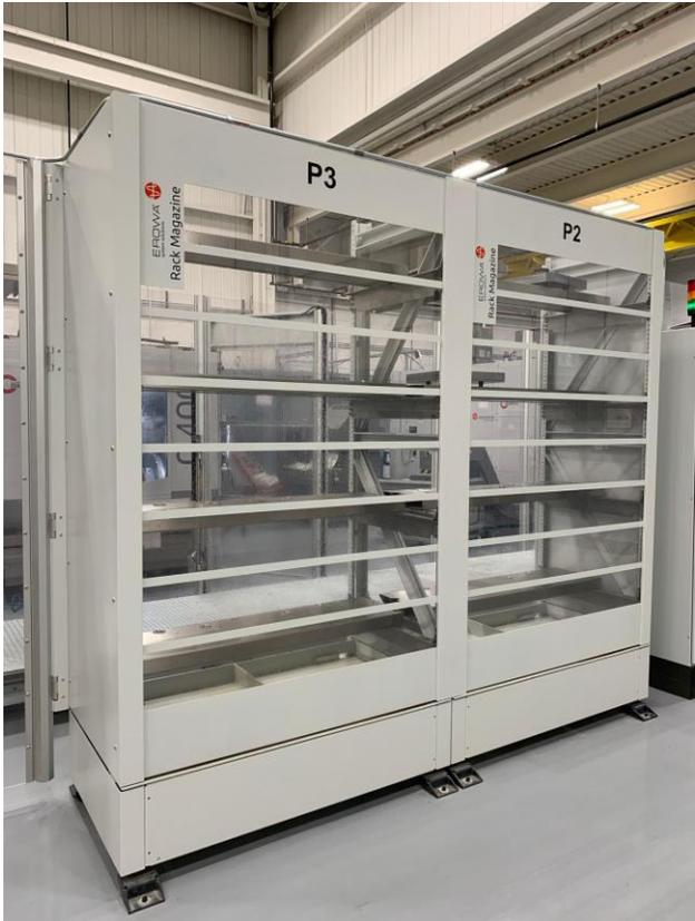
**Figure 4.9** EROWA® Rack magazine
