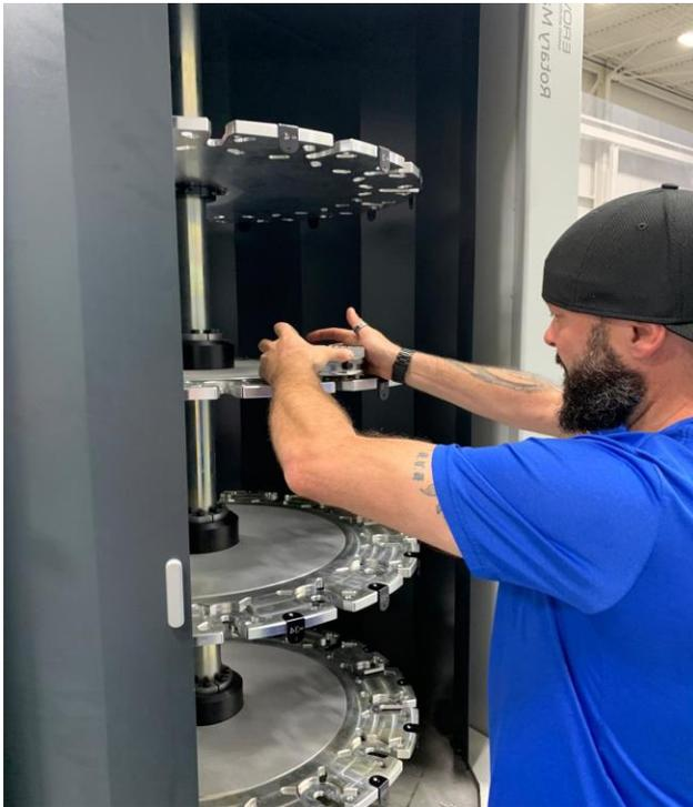
**Figure 4.11** SPM Automation Inc. operator loading EROWA® rotary magazine
