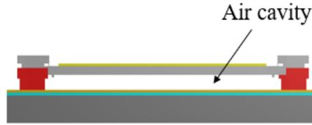
Figure 3.4: Cross-sectional view of the proposed micromirror Design 3 in MEMSPro using the PolyMUMPs fabrication layer sequence. Fabrication steps are described in detail in Chapter 5.
