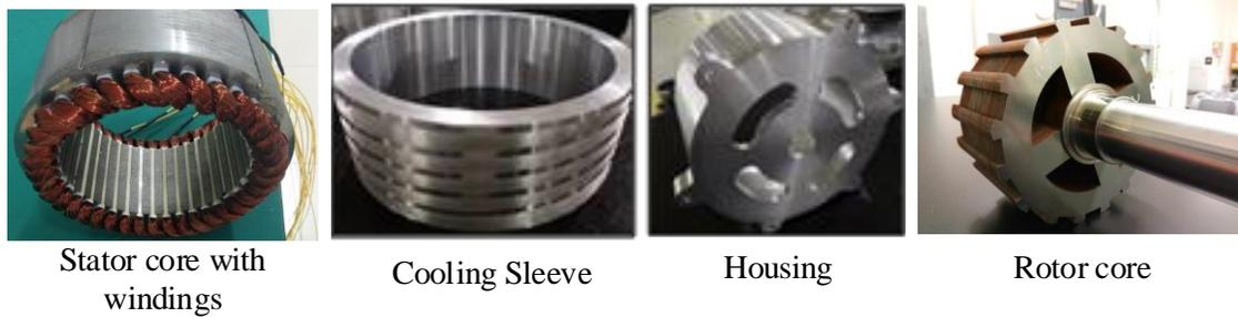
Figure 3.5 Several components of designed scale down SPMSM prototype.
