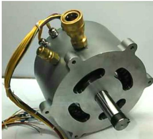
Figure 3.4 Designed scale down SPMSM prototype.
