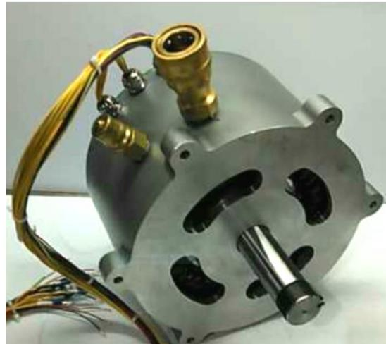
Figure 3.4 Designed scale down SPMSM prototype.
