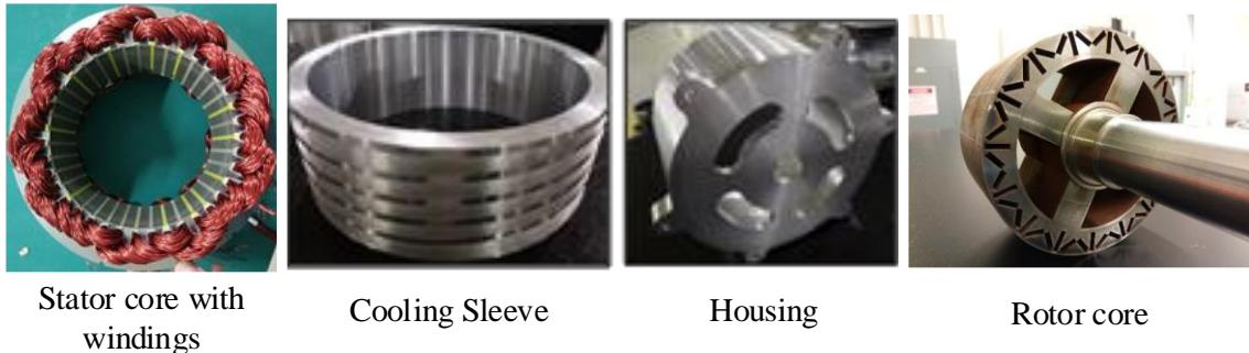
Figure 3.3 Several components of designed scale down IPMSM prototype.
