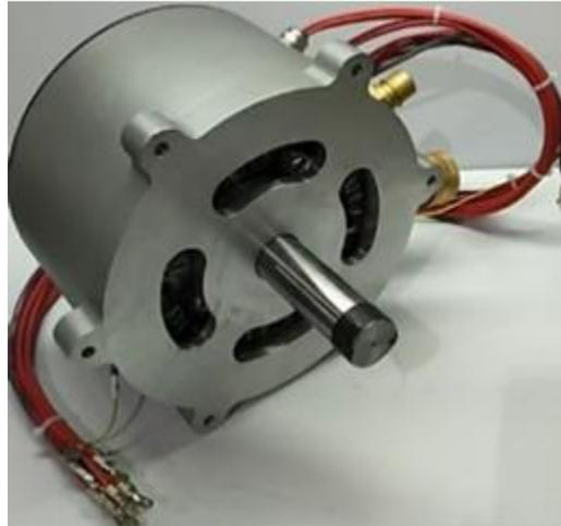
Figure 3.2 Designed scale down IPMSM prototype.
