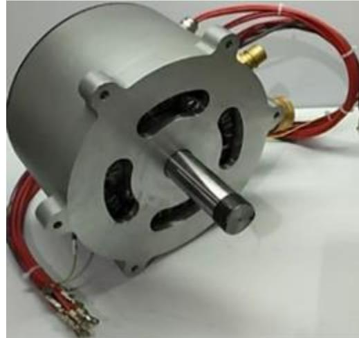
Figure 3.2 Designed scale down IPMSM prototype.
