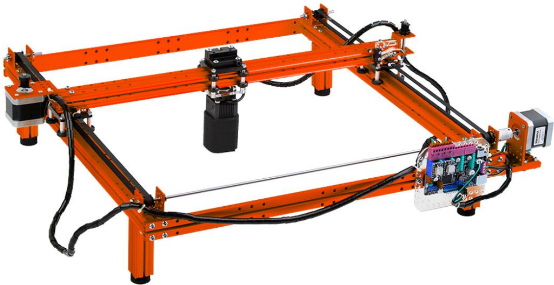
Figure 28 Laser setup with XY plane movement configuration
