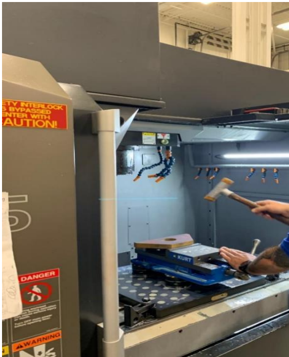
Figure 4.6 - SPM Automation Inc. operator placing raw material in CNC machine
