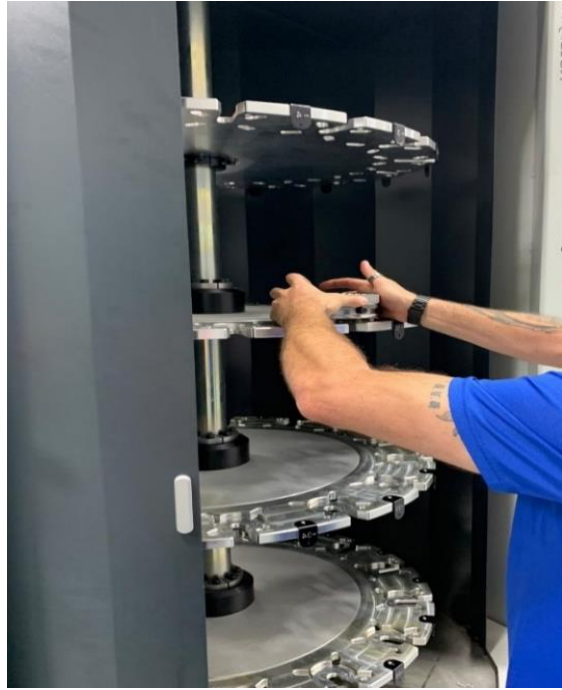
Figure 4.5 - SPM Automation Inc. operator loading EROWA® rotary magazine
