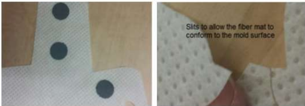
Figure 2.4 Fiber mats with complex geometrical shapes
