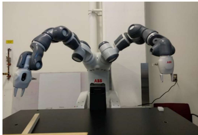
Figure 3.2 YUMI dual arm collaborative robot
