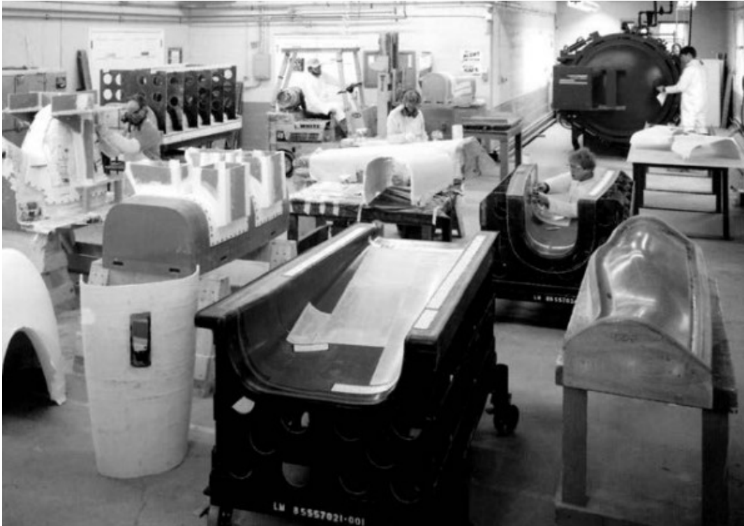
Figure 2.5 Master models and laminated molds (taken from [5])
