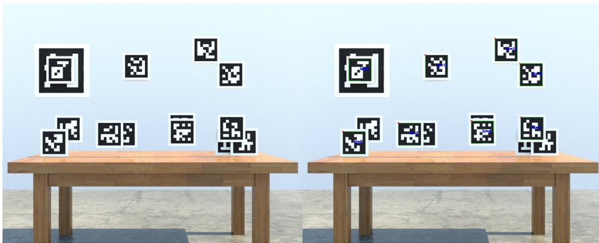
Figure 5.10: (Right) image produced by 3ds Max (Left) only fully visible markers were correctly detected
