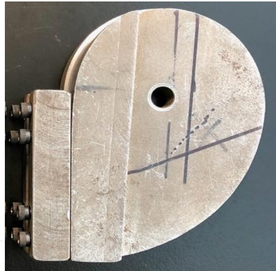
Figure 4.3. (Left) Tensile testing clamp patent design to maximize clamping pressure on magnet wire and mitigate breakage where 1 is the magnet wire, 2 is the clamp body, and 3 is the clamping member to secure the magnet wire over a large area [129]. (Right) Fabricated tensile testing clamp from [14] designed for use with rectangular cross section copper magnet wire and used for aluminum magnet wire in this study.
