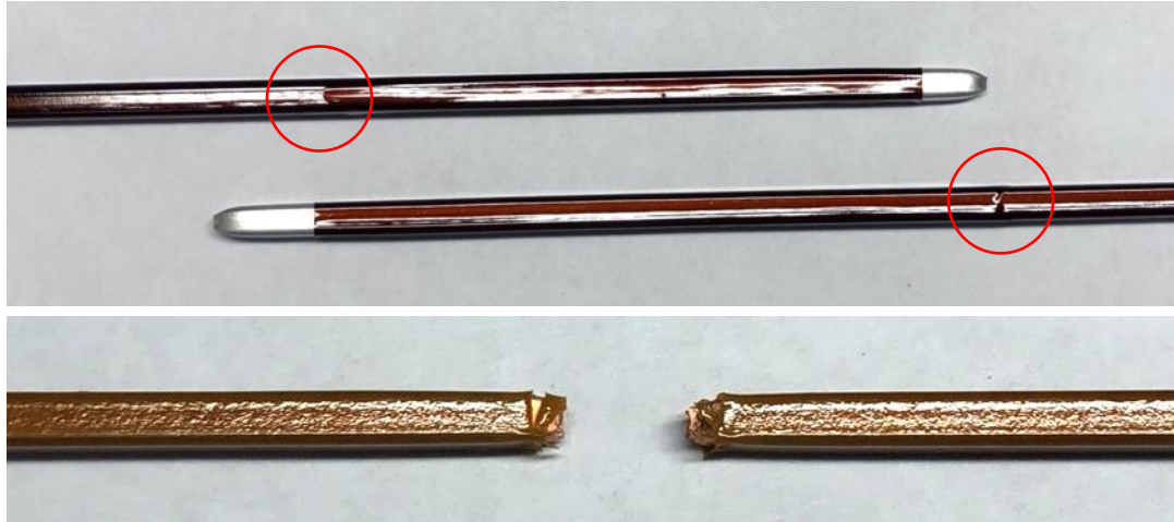
Figure 5.4. Fracture ends of aluminum wire elongated to failure highlighting a tube of delaminated insulation starting at the red circles and ending at the fracture end. Shrinkage of the insulation away from the aluminum wire fracture ends is also highlighted. Copper wire insulation does not see the same problem, remaining adhered up to the fracture end.
