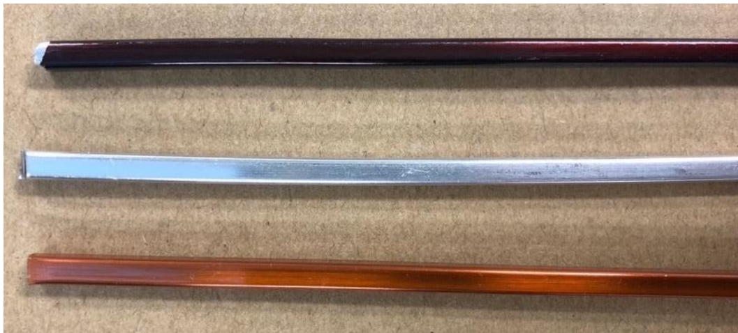
Figure 4.1. Magnet wire samples tested in this study: insulated aluminum (top), bare aluminum (middle), insulated copper (bottom).
