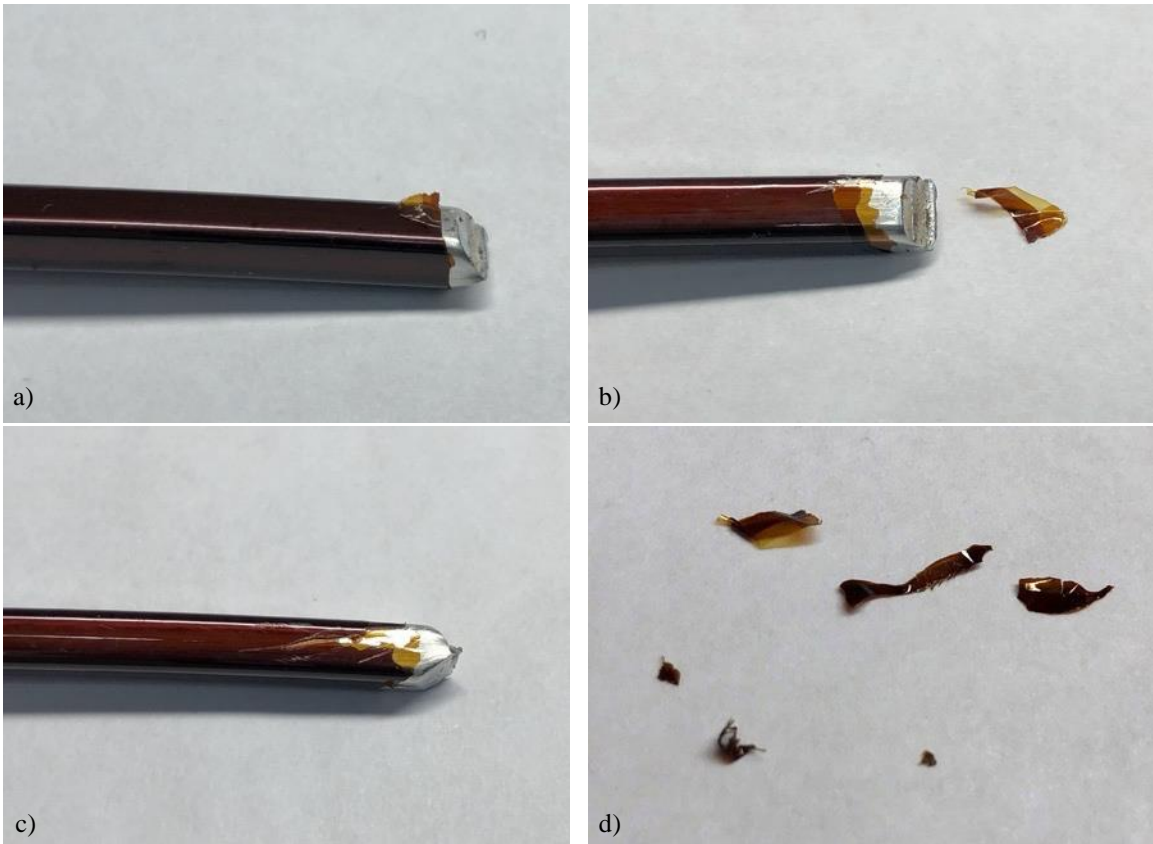
Figure 5.12. Peel test results for fresh, untested, insulated aluminum wire establishing baseline insulation adhesion. (a) A pull tab was able to be created with significant effort and damage to underlying aluminum. (b-c) Insulation adhesion was too strong to remove any significant amount of insulation with only small pieces breaking off (d).
