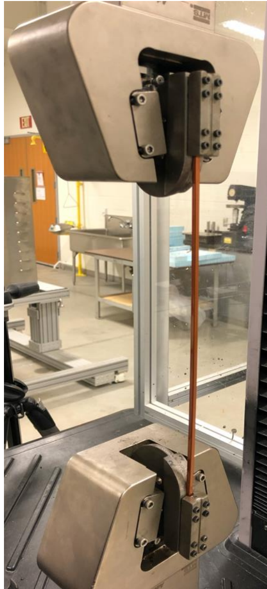
Figure 4.4. Alternate clamping method for aluminum and copper wires using only the clamping member of the tensile testing clamp to accommodate the shorter copper wires used in this study as well as to mitigate stress concentrations on aluminum wire at grip exit when used as intended.
