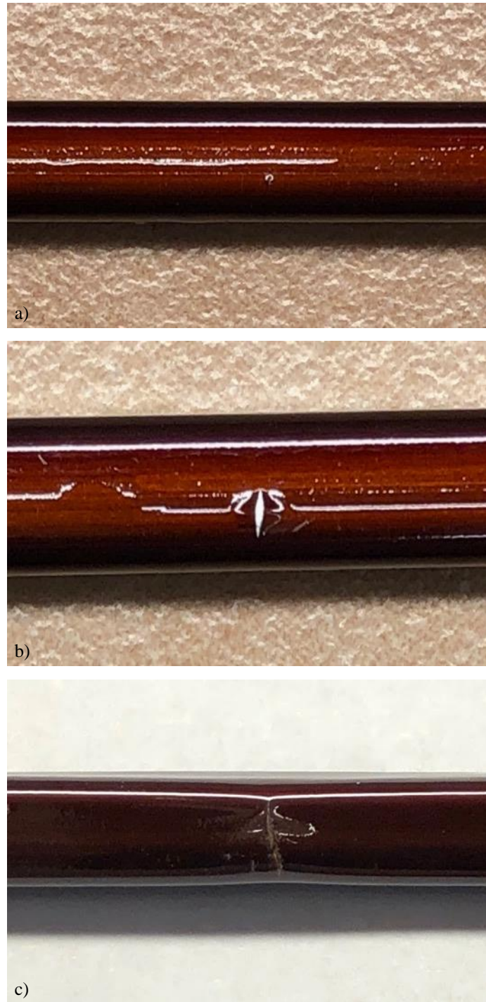
Figure 5.23. Aluminum insulation damage sustained during elongation to failure. (a) Small pinhole failure of insulation. (b) Less common, large split revealing the underlying conductor. (c) Example of gross insulation failure consisting of insulation split the width of the conductor and delamination zone around the fracture.
