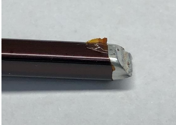
Figure 4.6. Example of peel test procedure on aluminum magnet wire where a knife is used to separate the insulation from the base conductor to create a pull tab for attempted insulation removal.
