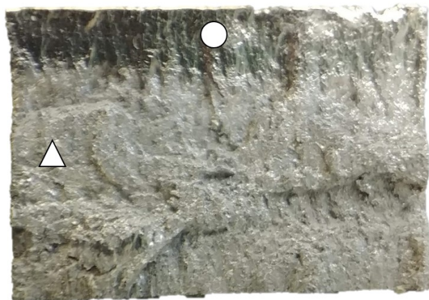
Figure 4.19: Photo of D2 side press fracture surface
