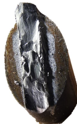
Figure 4.15: Typical Shear Compression Fracture Surface
