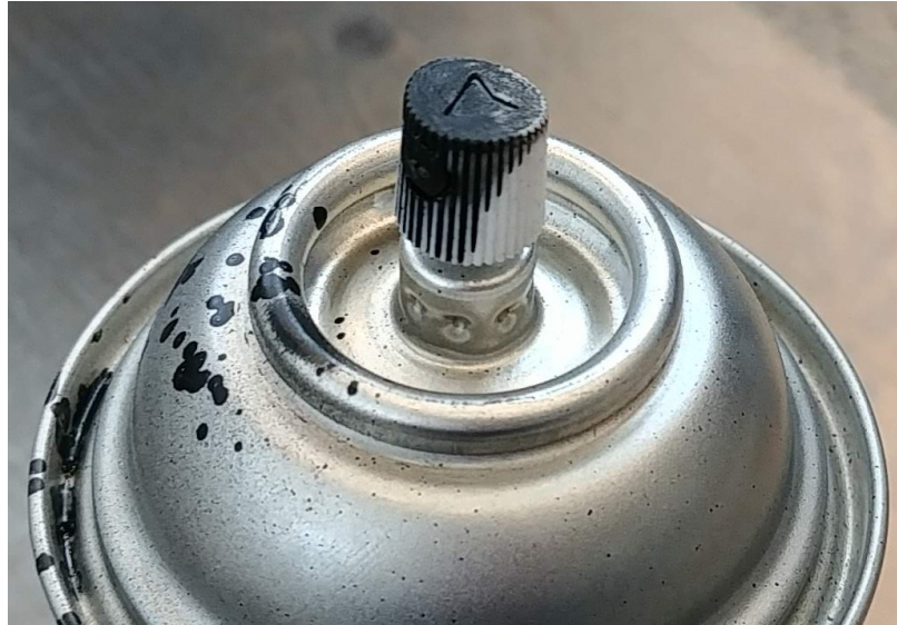
Figure 6.4: Image of spray nozzle used to achieve speckle pattern shown in Figure 6.5
