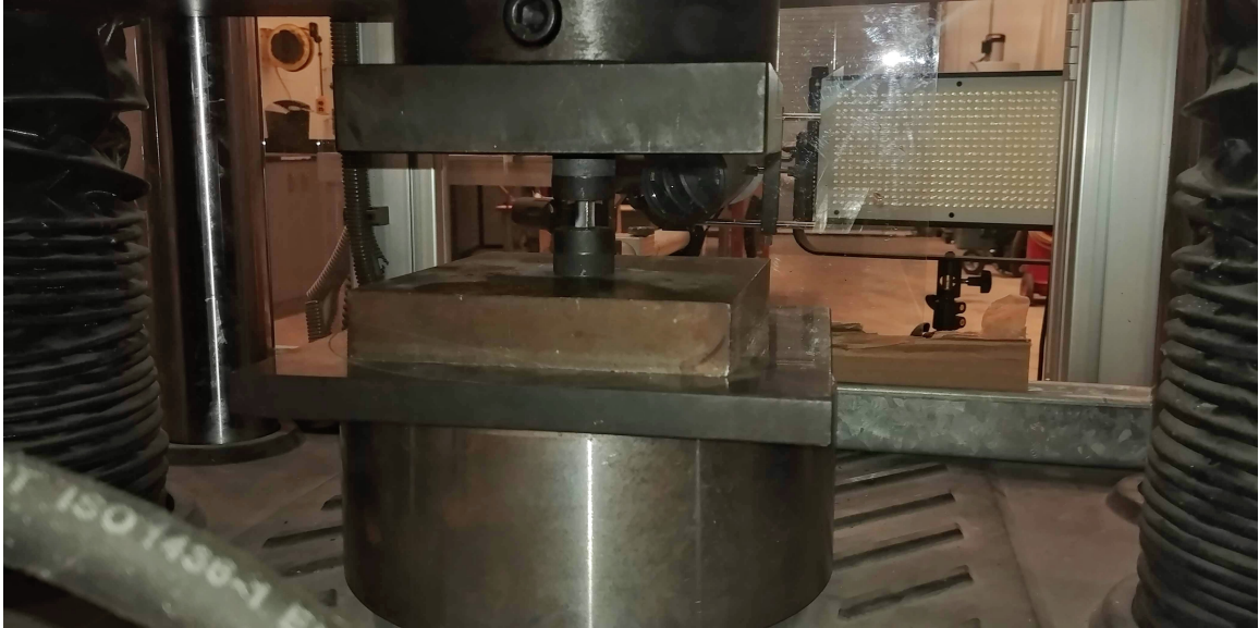
Figure 6.2: MTS Universal Testing Machine with 600kN load cell showing use of platens with compression sample
