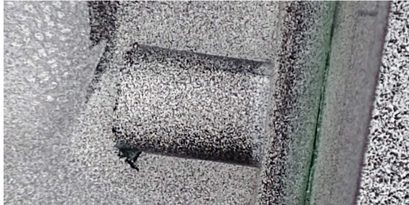
Figure 6.5: Image showing example speckle pattern applied to mechanical test samples
