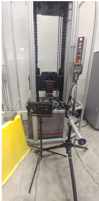
Figure 6.1: MTS Universal Testing Machine with 600kN load cell with camera and light for compression testing
