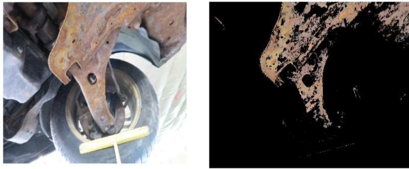
Figure 3.12: Red pixels corresponds to corroded area
