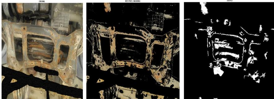
Figure 4.14: Corrosion detected and evaluated in DSCN5290.JPG
