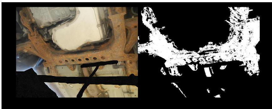
Figure 4.7: Defined boundaries of the detected corroded area
