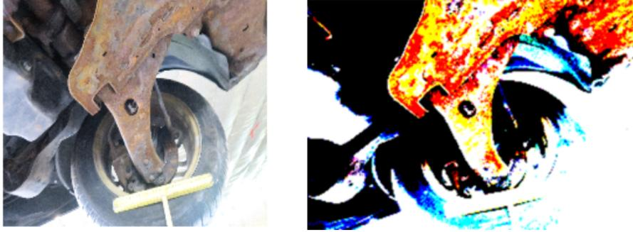
Figure 3.6: Corrosion detection using Otsu method
