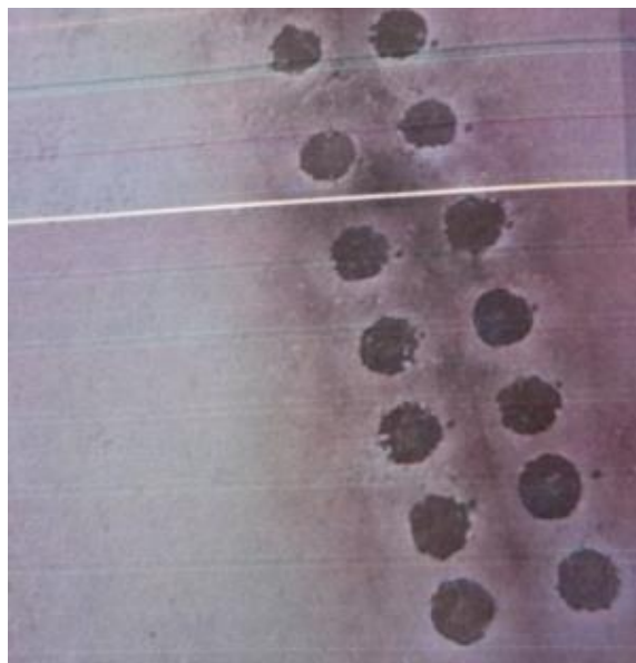
Figure 7.4: Zoomed in image of nitrocellulose filter with silver powder brushed along filter surface, captured using OASIS camera software. Craters displayed reproducibility among resulting LIBS spectra and visible ablation craters.
