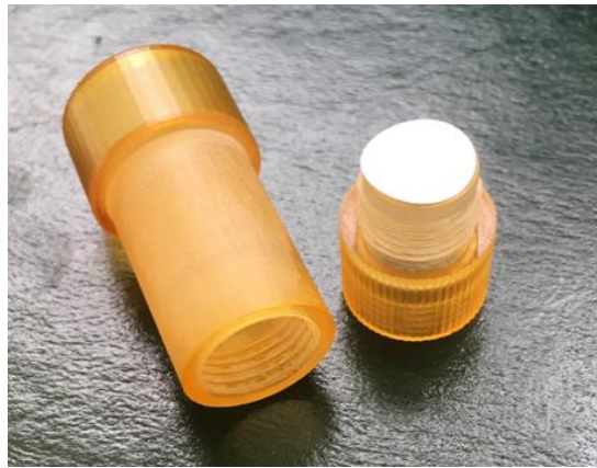
Figure 2.3: Insert unscrewed with filter paper placed on the base.
