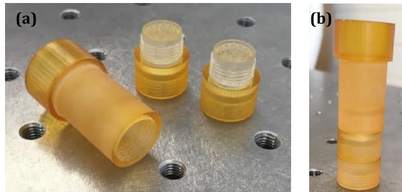
Figure 2.1: Custom fabricated centrifuge insert (a) disassembled (b) assembled.
