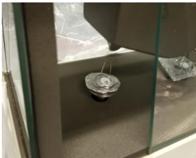
Figure 7.3: Silver coated nitrocellulose filters inserted into EA microbalance. Two filters are placed on the balances to provide a reference counterweight.
