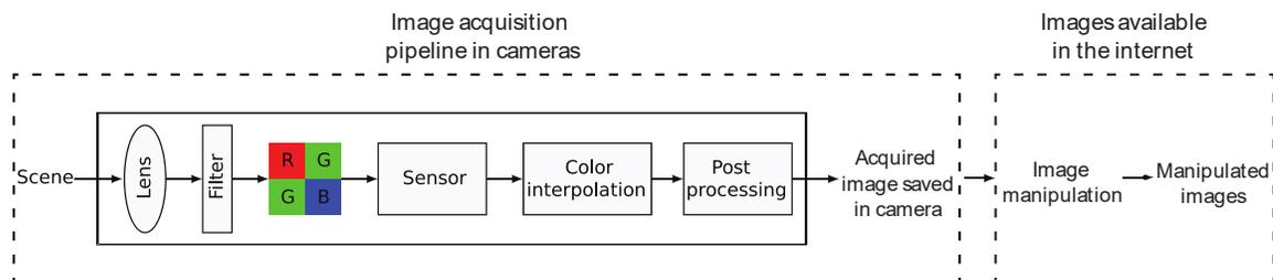
Figure 1: General acquisition pipeline of available digital images.
