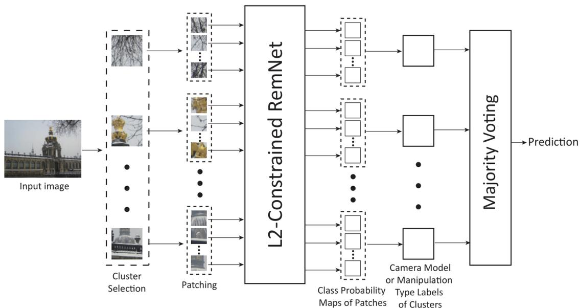
Figure 3: Schematic representation of the proposed method for CMI and image manipulation.
