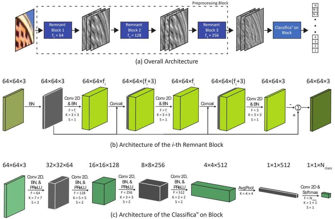
Figure 4: The architecture of our proposed RemNet. (a) Illustrates the overall architecture with three remnant blocks with one classification block. The architectures of the remnant and classification blocks are depicted in (b) and (c), respectively. In (b) and (c), AvgPool, BN, and Conv2D represent average pooling, batch normalization, and 2D convolution, respectively. The letters F, K, and S represent the number of filters, their kernel sizes, and
