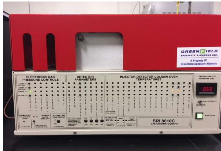
Figure 3.4 Gas chromatograph SRI 8610C and gas analysis experiment
