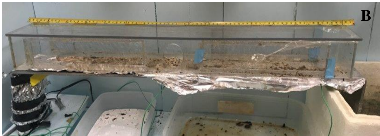
Figure 2.1. Images of the experimental set up inside the “environmental box” to maintain relative humidity conditions (A). The aluminum temperature gradient with aluminum foil liner and plexiglass arena placed on top (B).
