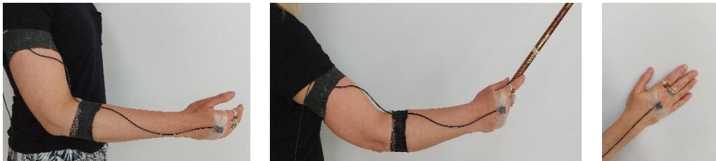
Figure 10. The accelerometer placement on the hands of the participant. Image used with permission from Dr. Nadia Azar.
