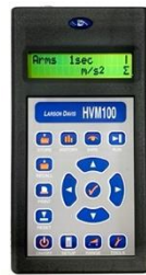
Figure 8. The HVM100 Human Vibration Meter. Image used with permission from Dr. Nadia Azar.
