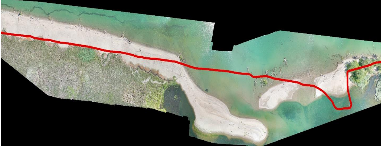
Figure 37: First UAV survey of this project (conducted in August 2020), compared to latest shoreline digitization (survey from July 2022).
