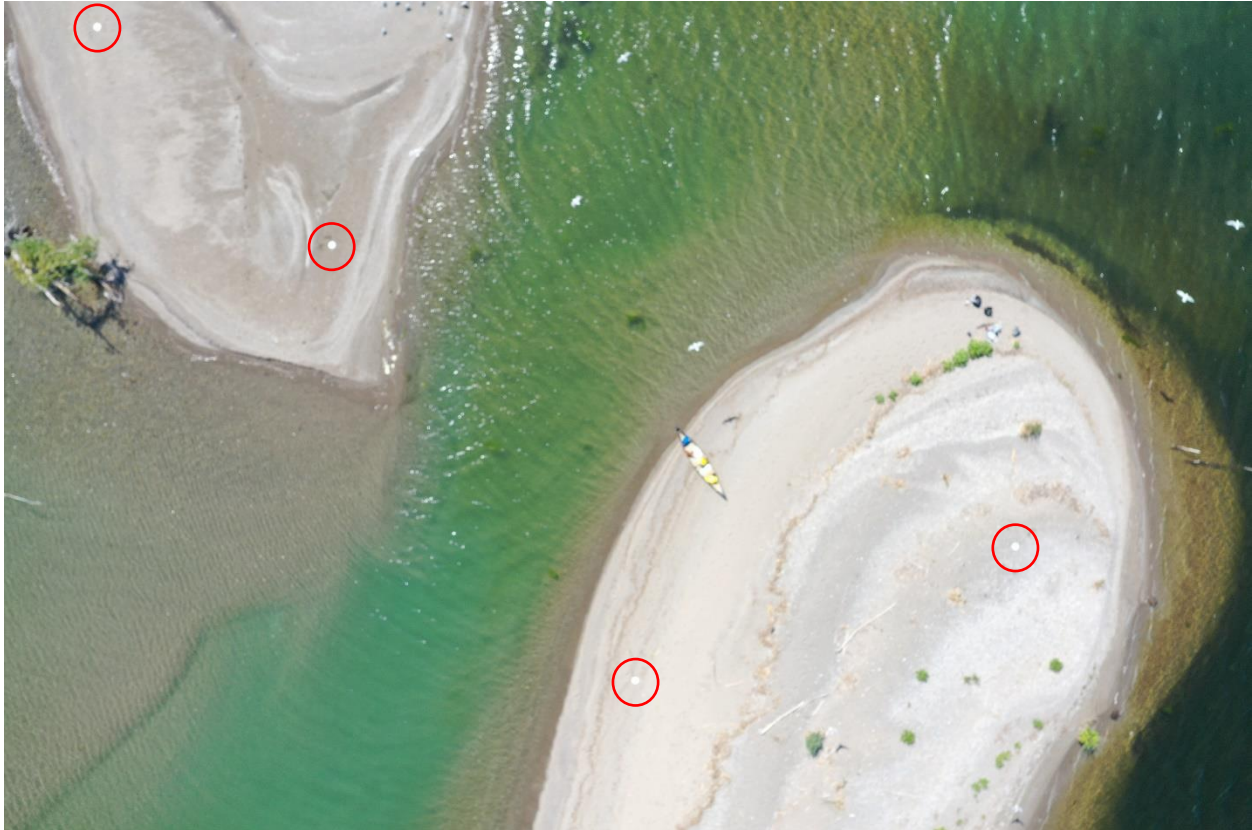
Figure 18: Ground Control Points (GCPs) in use during a survey at East Beach in August 2020. GCPs are assigned specific UTM coordinates using a Real Time Kinematic (RTK) capable GPS receiver, are georeferenced to increase the accuracy of the survey.
