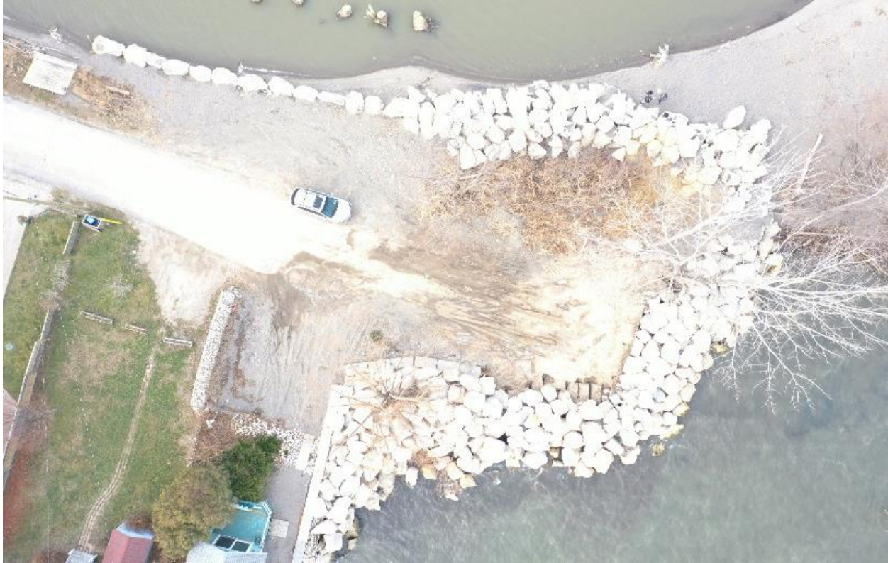
Figure 16: Rock revetment put in place by the City of Leamington in early November 2020.
