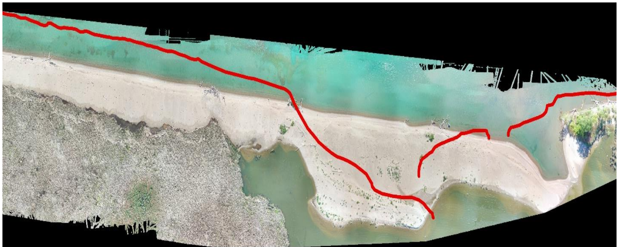
Figure 38: Last UAV survey of this project (conducted in July 2022), compared to first shoreline digitization (survey from August 2020).
