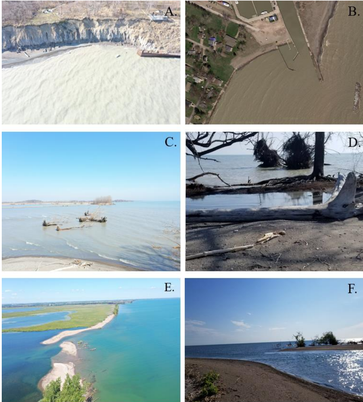
Figure 15: (A) Glacial bluffs located between Port Alma and Wheatley Harbor are the primary source of sediment in the Port Alma to Southeast Shoal littoral cell that supplies the eastern barrier of Point Pelee. (B) Wheatley Harbor and Jetty has trapped or removed \sim 500,000 \text{ m}^3 of sediment from the littoral cell causing an increased sediment deficit of the downdrift shorelines (Baird, 2007). (C) Hillman Beach was breached during the current high lake level period and has expanded rapidly and eroded most of the central and southern barrier. (D) Shoreline retreat at Hillman Beach has resulted in vegetation and tree loss. (E) and (F) show the aerial and ground view of the breach at East Beach.
