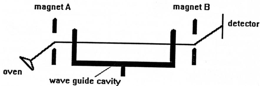
A typical atomic cesium clock is shown schematically in Figure 1 above. In the diagram magnets A and B have been rotated  $90^\circ$  about a vertical axis to show the tips of their poles.
