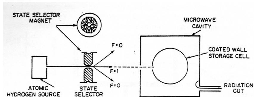
Figure 2. Schematic view of atomic hydrogen maser.
