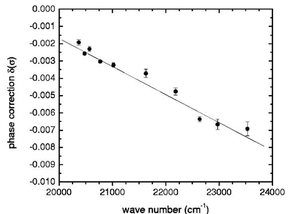
Fig. 3. Wave-number-dependent phase correction  $\delta(\sigma)$  resulting from reflections at the FP etalon mirrors, measured previously<sup>30</sup> by use of the method of virtual mirrors for seven different spacings. The results for  $\delta(\sigma)$  measured at 10 different wave numbers have been fitted to a straight line for interpolation.
