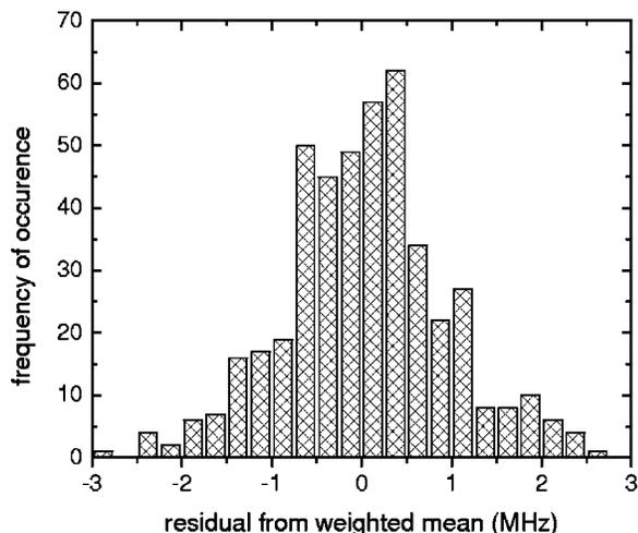
Fig. 4. Residuals for all wave-number measurements calculated by comparison of individual measurements with their weighted means. The standard deviation of the resulting histogram of 457 measurements is 0.97 MHz. This estimate of the measurement reproducibility is the dominant contribution to the final measurement uncertainty.
