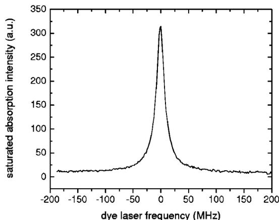
Fig. 2. Doppler-free saturated-absorption profile of the  $\text{Te}_2$  line at  $22\,634\text{ cm}^{-1}$ . The linewidth (FWHM) is 17 MHz. The cell temperature was  $502^\circ\text{C}$  corresponding to a vapor pressure of 91 Pa, and the pump beam and probe beam powers were approximately 100 mW and 10 mW, respectively.
